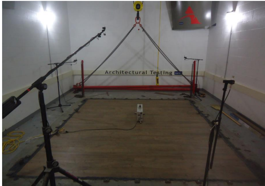
Source Room View of Test Specimen Installation
